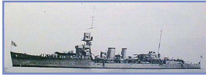
HMS Durban, built 29 May 1919, a 4,830 tons Light Cruiser of the Royal Navy with six 6" single-mounted guns (picture from Jane's Fighting Ships)
